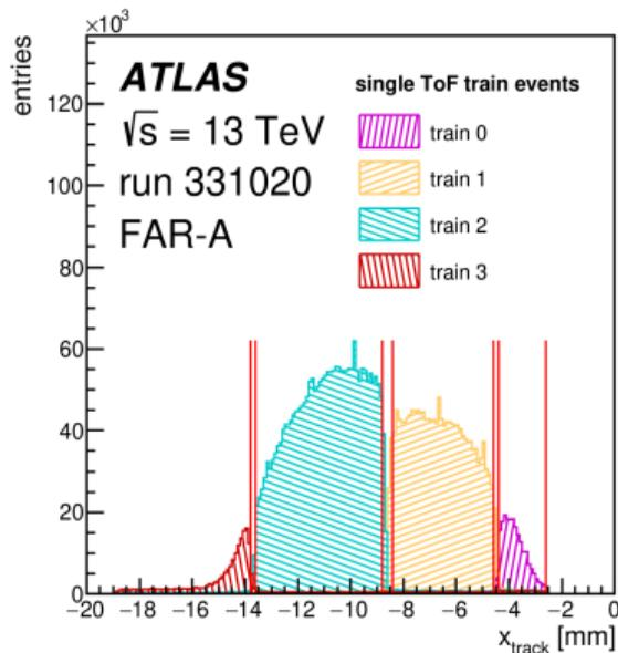
Distributions of local track  $x$ -coordinates in the AFP FAR station after applying the single-ToF-train selection in the AFP calibration stream run 331020. The red vertical lines indicate the chosen cuts that are used to define the acceptance of the trains.
