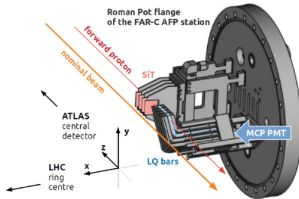
Detector package before installation (Run 2 design):
