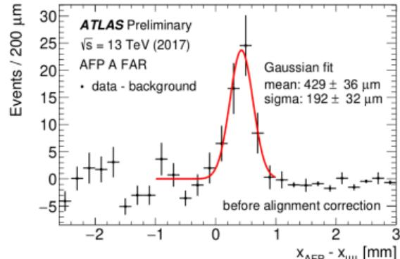
Illustration of the data-driven AFP global alignment method based on exclusive dimuon events:  $x_{A\text{FP}} - x_{\mu\mu}$  distribution after subtracting the background bin-by-bin. This distribution is attributed to signal events and is fitted to a Gaussian, the mean of which is taken to be the alignment off-set constant.
