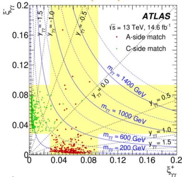
$(\xi_{\gamma\gamma}^+, \xi_{\gamma\gamma}^-)$  distribution of the selected data candidates after the full event selection in  $m_{\gamma\gamma}$  in [150,1600] GeV with  $m_{\gamma\gamma}$  contours (blue) and  $y_{\gamma\gamma}$  contours (black). The range of  $\xi_{\gamma\gamma}$  in which forward-proton matching is possible is indicated by the yellow rectangle for each side. Events passing the matching requirement on the A(C)-side are represented by the red dots (green triangles).
