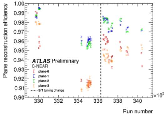
Efficiencies for each SiT plane in the C NEAR station, determined separately for each ATLAS run number. The step change in the vicinity of Run number 336000 corresponds to an adjustment of thresholds.
