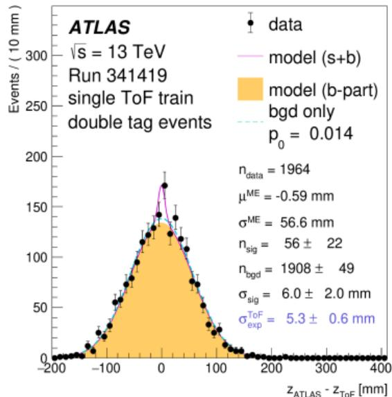
The  $z_{\text{ATLAS}} - z_{\text{ToF}}$  distributions measured in run 341419 (dots) using double-tagged events with the single-ToF-train condition. The fits of the sum of signal and background components are represented by solid lines. The background component is indicated by the filled area.
