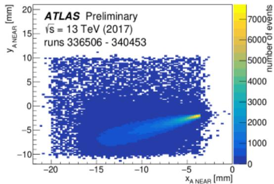
Occupancy of the AFP stations in terms of the  $(x, y)$  coordinates of track segments reconstructed from the loose dilepton selection for cases where there is exactly one segment reconstructed in a station. The colour-coded scale corresponds to the number of reconstructed track segments per bin.
