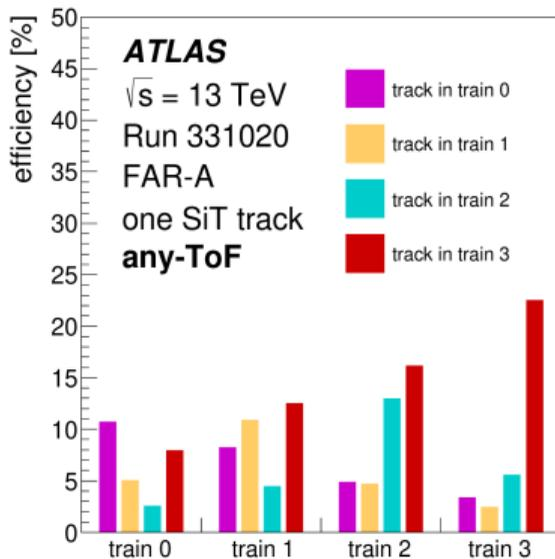
Efficiencies of ToF trains for the ATLAS run 331020 in the A-FAR AFP station. The data are required to contain exactly one reconstructed SiT track with no further constraints applied in the ToF.
