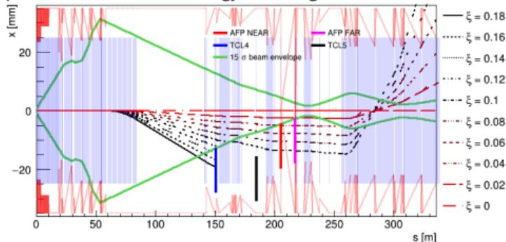
“Diffractive pattern” visible in the detectors; shape is due to LHC magnetic field:
