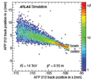
Positions of protons with given  $\xi$  and  $p_T$ ; depends on settings of LHC magnets:
