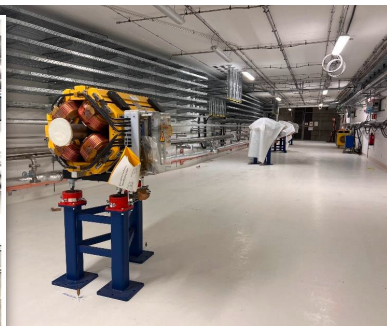
transport of the first quadrupole magnet in tunnel, Mar'24
